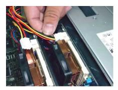
Connecting the power cable to the first *PL-P3/SMP*.
